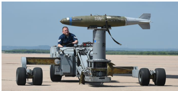
U.S. Air Force Tech. Sgt. Clayton Moore, 489th Maintenance Squadron weapons load crew member, transports a global positioning system-guided inert bomb unit using a jammer during the 2017 Global Strike Challenge at Dyess Air Force Base, Texas, June 13, 2017. The jammer is used to load and unload munitions into the B-1B Lancer. The GSC is a competition that showcases the world's best bombers, maintenance and security forces personnel units performing the Air Force Global Strike Command mission. (U.S. Air Force photo by Airman 1st Class Emily Copeland)
