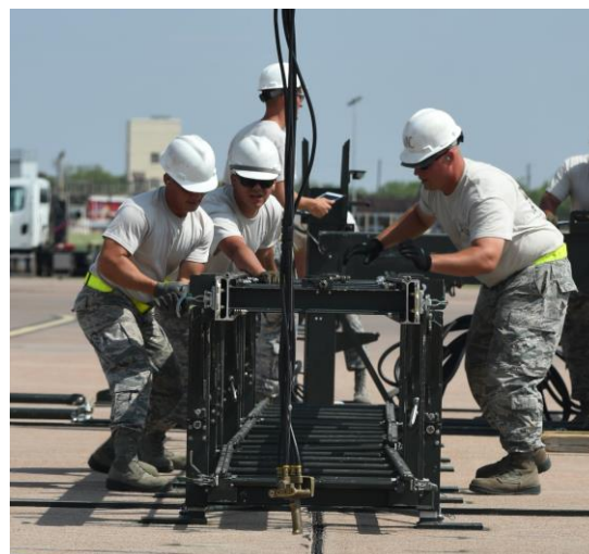
U.S. Air Force Airmen from the 7th Munitions Squadron, construct a munitions assembly conveyor during the 2017 Global Strike Challenge at Dyess Air Force Base, Texas, June 13, 2017. A munitions assembly conveyor is a mobile assembly line used to build bombs efficiently. GSC competitors are selected based upon available wing assets and determined by the unit's internal competitive team selection process. (U.S. Air Force photo by Airman 1st Class Emily Copeland)
