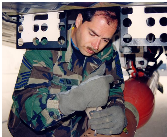
SMSgt Keith Hilton installing a WGU-25 guidance unit on a GBU-27 on the F-117A at Air Force Plant 42, Palmdale, CA around 1997
