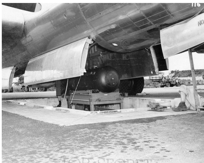
Hydraulic lift has raised the device about halfway into the bomb bay.
