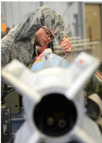
Airman 1st Class Kevin Gantt, 96th Aircraft Maintenance Unit Cobra 6 team member, tightens a bolt on a Guided Bomb Unit-12 during the quarterly weapons load competition inside the Weapons Load Training hanger on Barksdale Air Force Base, La., Jan. 9, 2015. Gantt was in charge of making sure all bombs were prepared and ready to load onto a B-52H Stratofortress U.S. Air Force photo/Senior Airman Joseph A. Pagán Jr.)
