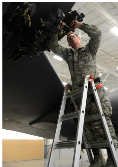
Senior Airman Tyler Branch, 96th Aircraft Maintenance Unit Cobra 6 team member, prepares a MAU-12 for a weapon load inside the Weapons Load Training hanger on Barksdale Air Force Base, La., Jan. 9, 2015. The MAU-12 ejector rack attaches to a pylon on the wing of a B-52H Stratofortress and can hold up to nine MAU-12s and their connecting bombs. (U.S. Air Force photo/Senior Airman Joseph A. Pagán Jr.)
